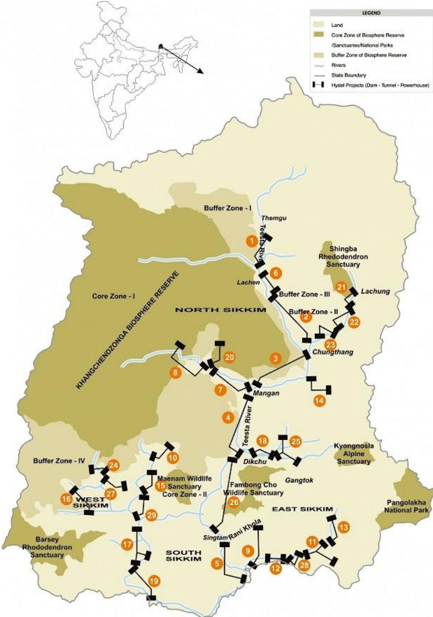
Figure 33: Plans for multiple large run-of-the-river hydropower projects in Sikkim will leave virtually no stretch of the Teesta river flowing free (Source: Sanctuary Asia / Vagholikar and Das, 2010).
